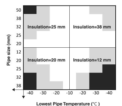
This table helps you in determining how many straight runs of cable you will need to protect your pipe. One run is equal to the length of the pipe. One run of 10ETR One run of 16ETR Two runs of 16ETR
